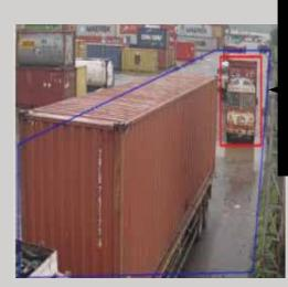
Notification generated for a stopped vehicle/ group of vehicles detected in the ROI for more than the specified threshold time.
